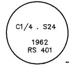
I FOUND A 1 1/2" IRON PIPE WITH A 3" OREGON STATE BOARD OF FORESTRY BRONZE CAP, (SEE T.C.S. MAP A-1034), LEANING, UNDERNEATH A LOG. I SAWED THE LOG OFF THE MONUMENT, STRAIGHTENED, AND ENCASED THE FOUND IRON PIPE IN AN IRREGULAR MASS OF CONCRETE.
