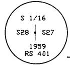
I FOUND A 1 1/2' IRON PIPE WITH A 3' D.S.B.F. BRONZE CAP (SEE T.C.S. MAP B-404). I ENCASED THE FOUND MONUMENT IN AN IRREGULAR MASS OF CONCRETE AND STONES.
