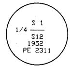
I FOUND A 1 1/2' IRON PIPE WITH A 3' D.S.B.F. BRONZE CAP, UP APPROXIMATELY 15', WITH DRIGINAL 14' X 10' X 7' STONE IN MOUND OF STONES SURROUNDING THE IRON PIPE. I ENCASED THE FOUND IRON PIPE AND BRASS CAP IN A MASS OF CONCRETE AND STONES. I PLACED THE ORIGINAL STONE MARKED \*1/4\* ON THE NORTH SIDE OF THE IRON PIPE MONUMENT.
