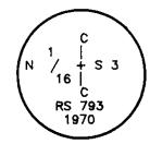
I found a 2" iron pipe with a 3" Tillamook County Surveyors Brass Cap, (see T.C.S. Rewitness Card #349), I set an 8" cast iron monument case around the found monument and encased in concrete, flush with the surface of the pavement.
