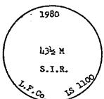
From which scribed: 9" hemlock bears S 10° W 30.45 feet; scribed "SIR 432M", screw nail, lead washer, yellow aluminum section marker plate
