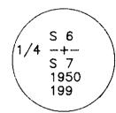
I Found a 1 1/2" iron pipe with a 3" O.S.B.F. Bronze Cap. I encased the found I.P. in a 10" concrete cylinder .
