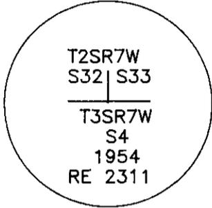
I found a 1 1/2" iron pipe with a 3" O. S. B. F. Bronze Cap, (see T.C.S. Rewitness Book 2 at Page 176). I encased the found iron pipe in a 10" concrete cylinder.
