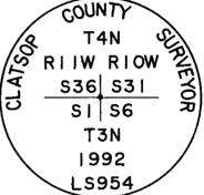
Top 38" below the ground surface for a subsurface monument. placed 8" of dirt over the cap.
