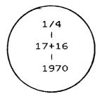
I found a 1 1/4" iron rod with a 3" Tillamook County Surveyors brass cap, (see Tillamook County Surveyors rewitness card #613). I set a 10" cast iron monument case around the found iron rod with brass cap, and encased in concrete.
