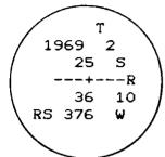
I found a 3/4" iron pipe 5' long with a 3" Crown Zellerbach brass cap 36" high in pile of logs. I sawed the logs out and lowered the cap to approximately 4" above the ground and encased in a 10" concrete cylinder. (See Tillamook County Surveyors rewitness book 3 page 301).
