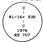
I found the O.S.B.F. 1 1/2" iron pipe with 3" bronze cap set in 1976, (See Tillamook County Surveyors map #B-749), and encased in a 10" concrete cylinder.
