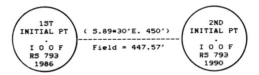
I set a 1 1/2" iron pipe with 3" Tillamook County Surveyors brass cap in 10" concrete cylinder at the position of a found 6"x9"x22" stone marked "X" as called for in Tillamook County Surveyors Survey book 53 at page 400.
