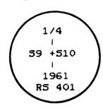
I set a 10" concrete cylinder around found 0.5.B.F. 1 1/2" iron pipe with 3" bronze cap set in 1961, (See Tillamook County Surveyors map #B-437).
