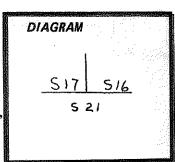
A dead fir snag 50 ins diam bears N84°W 29 1ks mkt T6S R10W S17 BT. A willow 4 ins diam bears S72°E 47 lks mkt T6S R10W S21 BT. Raised a mound of stone around corner 4 ft. at base, 2 ft. high.
