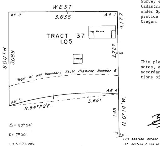
This plat represents a retracement and reestablishment of a portion of the subdivisional lines of T. 1 S., R. 8 W., Willamette Meridian, Oregon, designed to restore the corners in their true original location according to the best available evidence; the subdivision of section 7 and survey of Tract No. 37.
